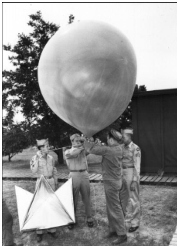
Figure 1. A neoprene weather balloon and a 1947-era rawin radar target.
