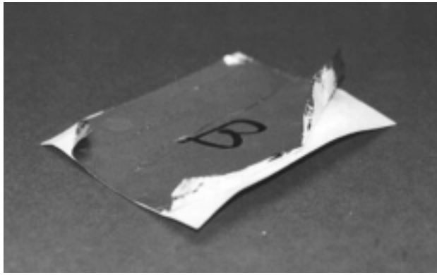
Figure 6. A partially delaminated piece of simulated rawin radar-target laminate made from aluminum foil and paper. Portions of similar materials depicted in the Fort Worth, Texas, photos had also separated from each other. Most of that damage probably occurred when the target impacted the ground and was subsequently dragged over vegetation and exposed rocks by the remaining inflated balloons in the Mogul Flight 4 or equivalent balloon train.
